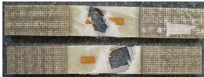
Fig. 95 MD coupons at 60° off-axis tested at R=-1.
