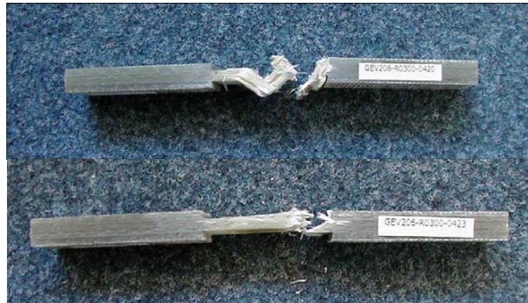
Fig. 11 Typically buckled (top) and valid (bottom) failure modes of the UD on-axis coupon, under R=10 fatigue.
